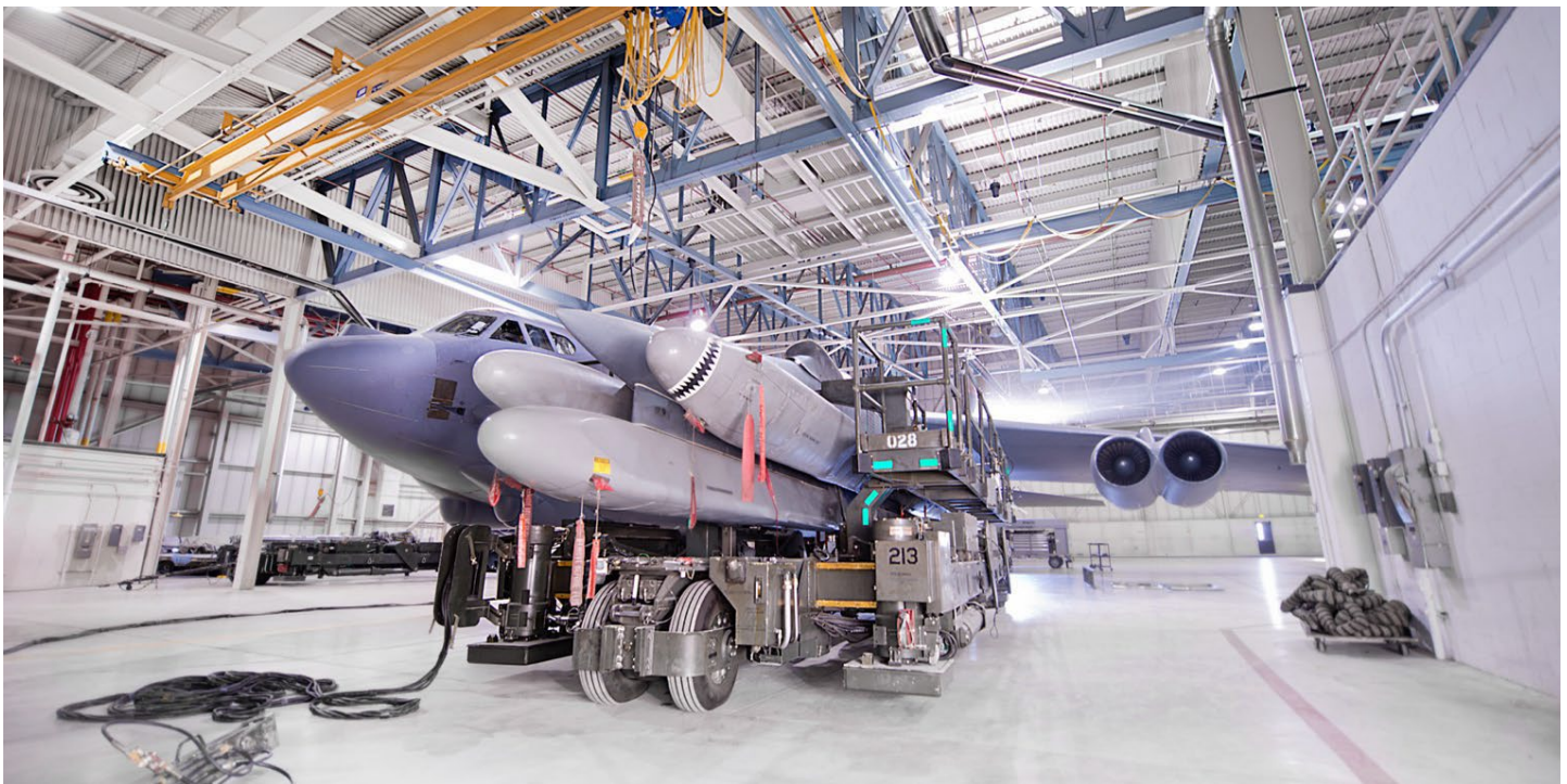
5 th Aircraft Maintenance Squadron load crews prepare to load an AGM-86B air-cruise launch missile trainer onto a B-52H Stratofortress at Minot Air Force Base, N.D., Feb. 26, 2014. As part of Air Force Global Strike Command, load crews work endlessly to preserve our nation's security by providing combat-ready forces for nuclear deterrence and global strike operations. (U.S. Air Force photo/Tech Sgt. Aaron D. Allmon II)
